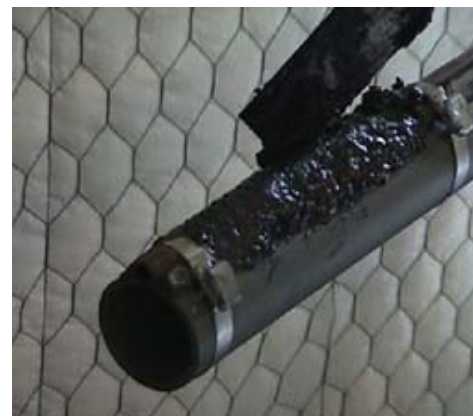
Typical hand trowel application
