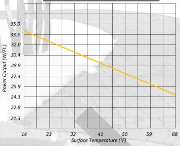
The following graph indicates the cable performance when buried in concrete. For other conditions, refer to the Factors Table shown below.
